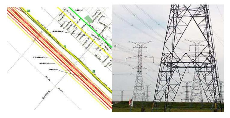
The red lines are directly below the high tension wires. The radiation from AC power drops off very rapidly as you move away from the lines but levels off at  $0.01 \text{mW/cm}^2$  over highway 407 and the adjacent residential neighborhood. The green line, indicating a level of  $1 \mu \text{W/cm}^2$  begins at 1.5km from the power lines.
